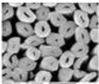
Fig. 6 Cross-sectional views of Thermolite® fibers [54]
