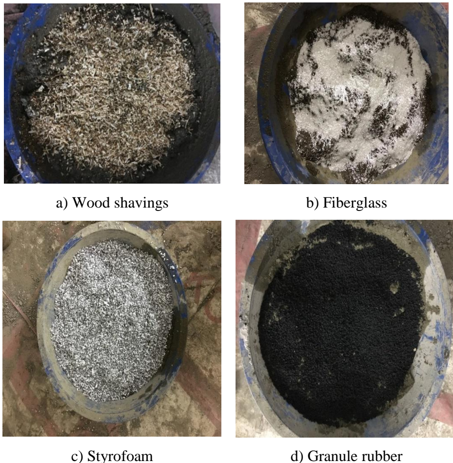
Figure 6. Various heat-insulated materials for the front wall part.
