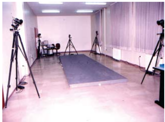
Fig. 1. A three-dimensional quantitative gait analysis laboratory.
