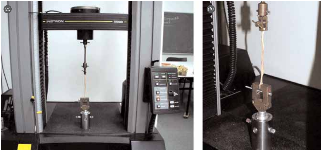
Fig 4. (a) The Instron® device and (b) the tendon strength measuring. [Color figure can be viewed in the online issue, which is available at www.aott.org.tr ]
