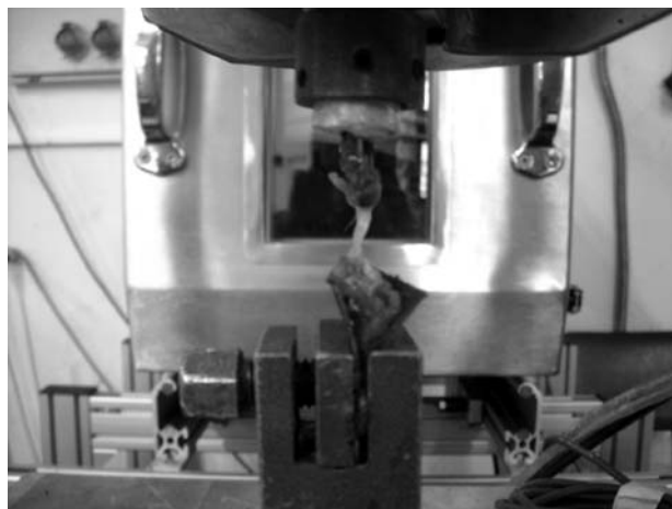
Fig. 2. Mechanical testing of the specimen. Tendon lengthening just before the rupture. [Color figure can be viewed in the online issue, which is available at www.aott.org.tr ]
