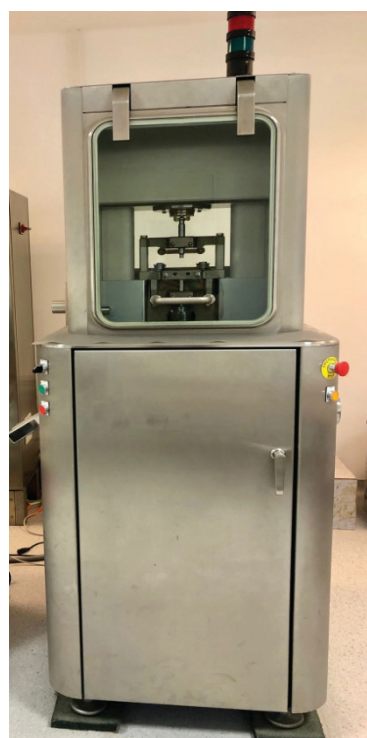
Figure 1. Image of Stylcam 200R; mechanical rotary cam compaction simulator (Jiwa, 2020).
