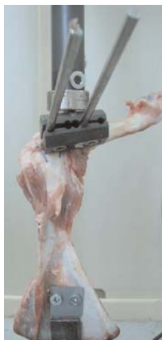
Fig. 3. The photograph of cadaveric sheep shoulder on Instron 8874 machine. [Color figure can be viewed in the online issue, which is available at www.aott.org.tr ]
