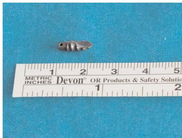
**Fig. 1.** Photograph of an Ti-6Al-4V anchor. [Color figure can be viewed in the online issue, which is available at [www.aott.org.tr](http://www.aott.org.tr)]
