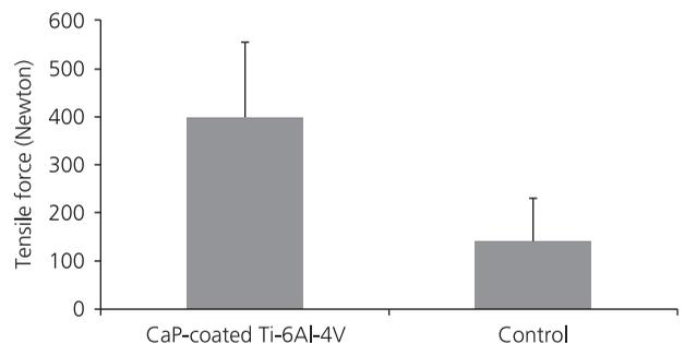
**Fig. 4.** Biomechanical test results of CaP-coated and uncoated anchor screws following *in vitro* tests.
