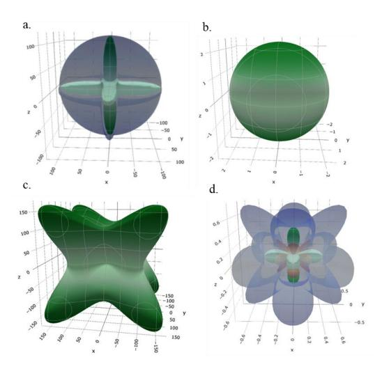
Figure 1. Three-dimensional elastic anisotropy; (a) Shear modulus(G), (b) Linear compressibility ( $\beta$ ), (c) Young's modulus(E), (d)Poisson's ratio ( $\upsilon$ )
