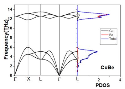
Figure 3. Phonon dispersion curves and partial PDOS of the CuBe compound
