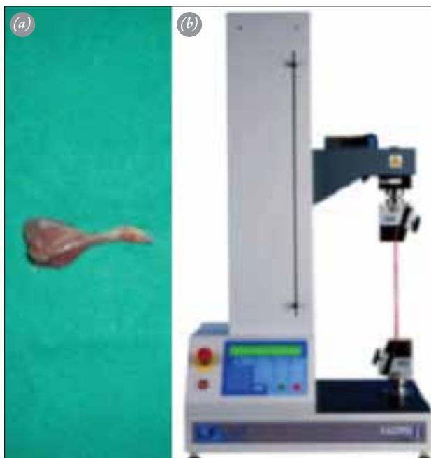
**Fig. 3.** (a) The Achilles tendon that was excised together with the calcaneus and gastrocnemius muscle. (b) Tensile testing machine. [Color figure can be viewed in the online issue, which is available at [www.aott.org.tr](http://www.aott.org.tr)]
