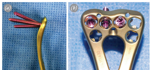
Fig. 2. Photograph showing the locking between screws and plate at three different angles; 15° upward, 0° and 15° downward. (a) Photograph showing good fit of the three differently-angled screw heads with the threads of plate holes. The leverage within available angle does not break the locking mechanism between plate and screws (b). [Color figures can be viewed in the online issue, which is available at www.aott.org.tr ]
