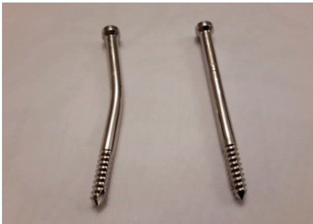
Fig. 3. Post- (left) and pre- (right) bending of 5-mm unthreaded stainless steel locking screws. [Color figure can be viewed in the online issue, which is available at www.aott.org.tr ]
