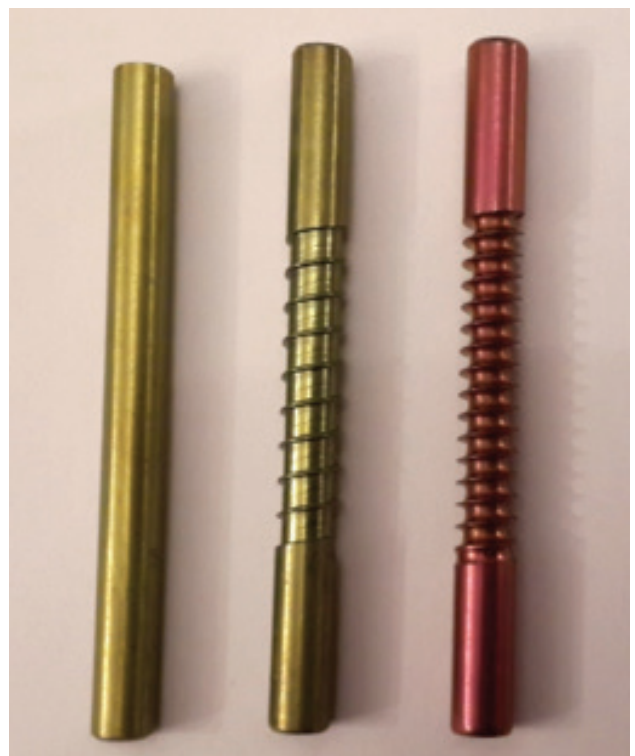
Fig. 1. 5-mm unthreaded, low threaded, and high threaded titanium locking screws. [Color figure can be viewed in the online issue, which is available at www.aott.org.tr ]
