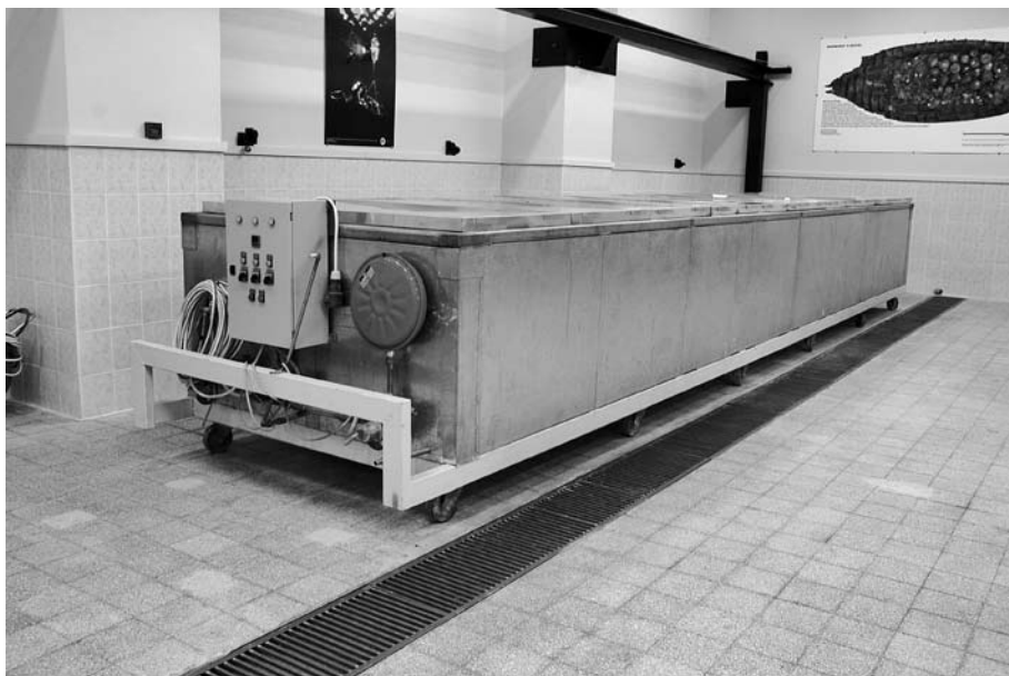
Fig. 11 Stainless steel pools manufactured for the conservation of the shipwrecks (Photo: N. Kılıç).
