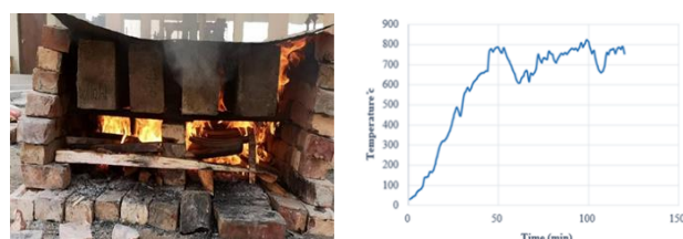
a). Damage by fire b). Temperature and time
