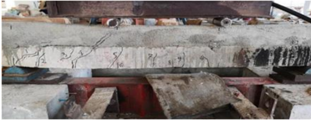
b). single layer Ferro cement strengthened beam
