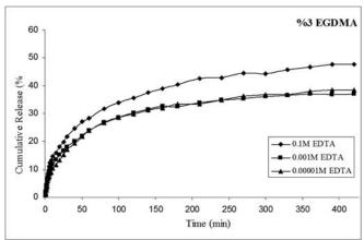
Figure 2. The effect of chelating agent on the cumulative release of gentamicin as a function of time from 50 wt % PEG-DA in the presence of 3 wt % EGDMA.
