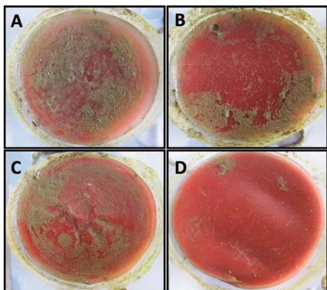
Figure 3. Cu<sub>2</sub>O gels in order of increasing concentrations. (A) 0.1 g Cu<sub>2</sub>O, (B) 0.2 g Cu<sub>2</sub>O, (C) 0.3 g Cu<sub>2</sub>O, (D) 0.4 g Cu<sub>2</sub>O.
