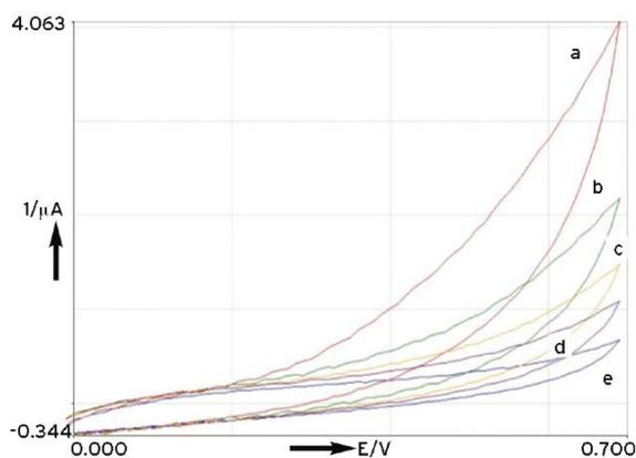
**Figure 1.** CVs of the mushroom (*Agaricus bisporus*) tissue homogenated based biosensor. (Phosphate buffer; pH 7.0, 50 mM, T: 30°C) (from a to e: baseline, 1.0, 2.5, 5.0, and 10.0 mM ethanol). The amount of homogenate, gelatine and percentage of glutaraldehyde were kept constant at 200.0 mg, 5.0 mg, and 2.5%, respectively. Scan rate is 25 mVs<sup>-1</sup> and potentials referred to Ag/AgCl reference electrode.
