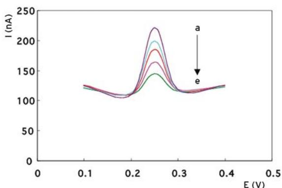
**Figure 3.** Differential pulse voltammograms obtained for different ethanol concentrations. (Phosphate buffer; pH 7.0, 50mM, T: 30°C) (from a to e: 1.0, 2.5, 5.0, 7.5 and 10.0 mM ethanol). The amount of homogenate, gelatine and percentage of glutaraldehyde were kept constant at 200.0 mg, 5.0 mg, and 2.5%, respectively.
