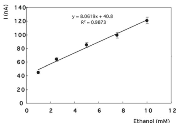
**Figure 4.** Calibration curve of the biosensor. (Phosphate buffer; pH 7.0, 50 mM). The amount of the mushroom tissue, the percentage of glutaraldehyde, gelatin amount and temperature were kept constant at 200 mg, 2.5%, 5 mg and 30°C, respectively.
