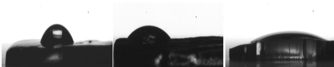
**Figure 1.** Photographs showing interactions of different solvents with CaAlg gels (a) paraffin (b) ethylene glycol (c) water.
