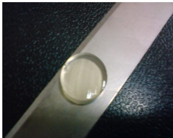
**Figure 2.** CaAlg gels in disc form and their slices made from 1.5% alginate solution and 1.75 X  $\text{CaCO}_3$ .
