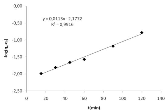
**Figure 5.** Linear transforms of  $\log(q_e - q_t)$  versus time at various temperatures for the adsorption of Cr(VI): 600 mg.dm<sup>-3</sup> Cr(VI); pH:2.0.
