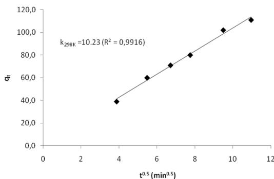
**Figure 4.** Effect of pore diffusion studies of Cr(VI) adsorption onto poly(EGDMA-VIM) beads: 25°C; pH:2.0; 600 mg.dm<sup>-3</sup> Cr(VI).
