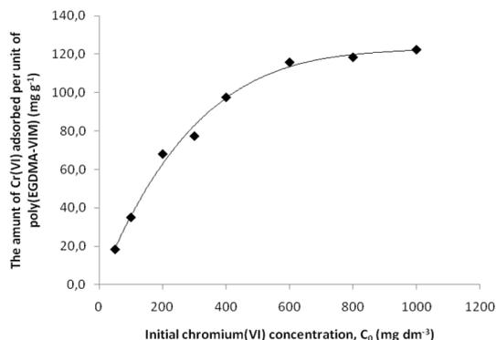
**Figure 3.** Effect of initial Cr(VI) concentration onto poly(EGDMA-VIM) beads: 25°C; pH:2.0; 180 min.
