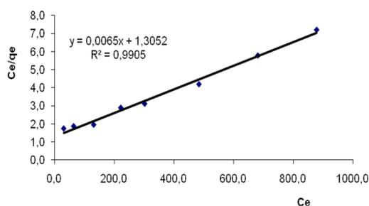
**Figure 7.** Establishment of the Langmuir monolayer adsorption constant for the adsorption of Cr(VI) at 298 K onto poly(EGDMA-VIM).
