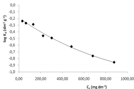
**Figure 8.** Distribution coefficients of Cr(VI) as a function of equilibrium solution concentration at pH 2 and 298 K.
