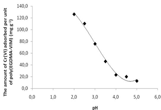
**Figure 2.** Effect of pH on adsorption of poly(EGDMA-VIM) beads: 600 mg dm<sup>-3</sup> Cr(VI); 25 °C; 180 min.
