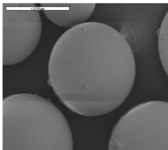
Figure 1. SEM photograph of poly(EGDMA-VIM) beads.
