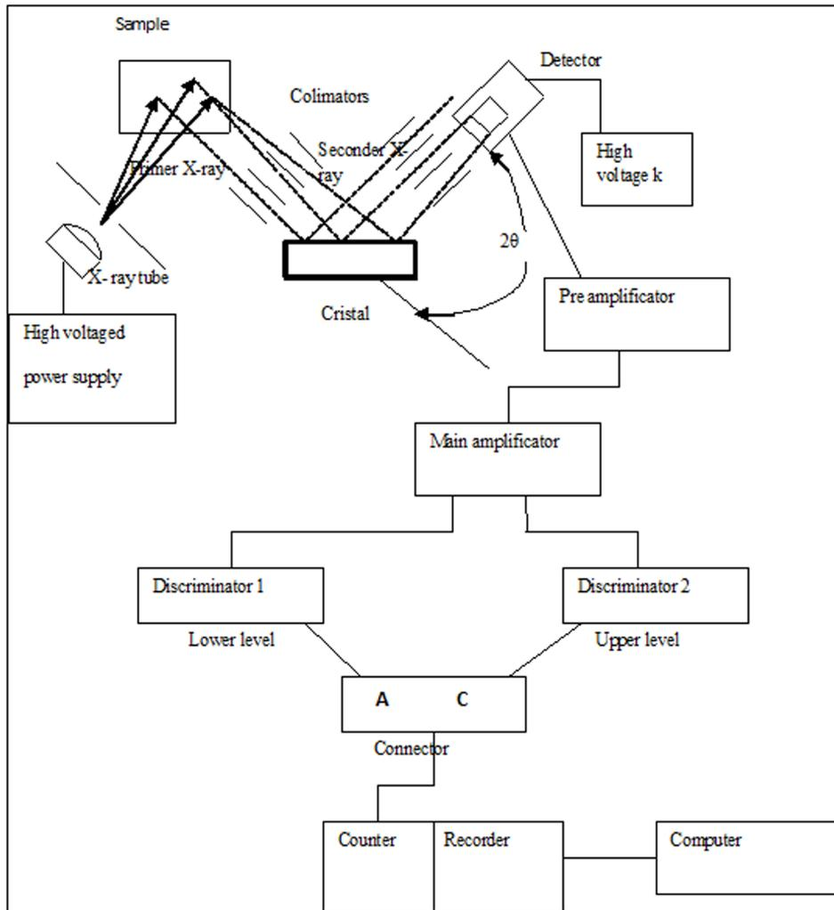
Figure 1. The used WDXRF system and its units
