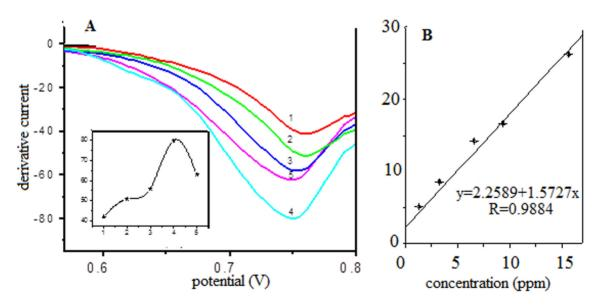
**Figure 3.** A) Derived voltammograms of MCPE electrode prepared with different particles size of graphite powder (1) 0.5-0.2 mm; (2) 0.2-0.16 mm; (3) 0.16-0.09 mm; (4) 0.09-0.071 mm; (5) 0.071-0.056 mm, with phenol concentration 3.3 ppm, in phosphate buffer 0.1 M ( pH 7), scan rate 50 mV/s, B) Calibration curve obtained at potential 0.78 V for 0.09-0.071 mm granulometry.
