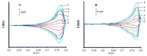
**Figure 2.** Cyclic voltammograms in 0.1 M phosphate buffer pH 7, scan rate = 50 mV/s. using CPE (A) and MCPE (B), in different phenol concentrations (0) buffer, (1) 1.4 ppm, (2) 3.3 ppm ; (3) 6.6 ppm ; (4) 9.4 ppm; (5) 9.4 ppm; using CPEM in the same phenol concentrations.
