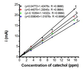
**Figure 4.** Calibration curves of CPEM using a.b.c.d section as modifier, E = 0.4 V, scan rate 50 mV/s.
