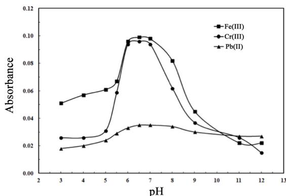
**Figure 1.** Effect of pH on the CPE of 200 µg L<sup>-1</sup> Pb(II), Fe(III) and Cr(III). Other conditions: sample volume 25 mL, 0.04% (w/v) Magneson I, 0.2% (v/v) Triton X-114, dilution solvent 0.1 mol L<sup>-1</sup> HNO<sub>3</sub> in ethanol, temperature 70 °C, time 45 min.
