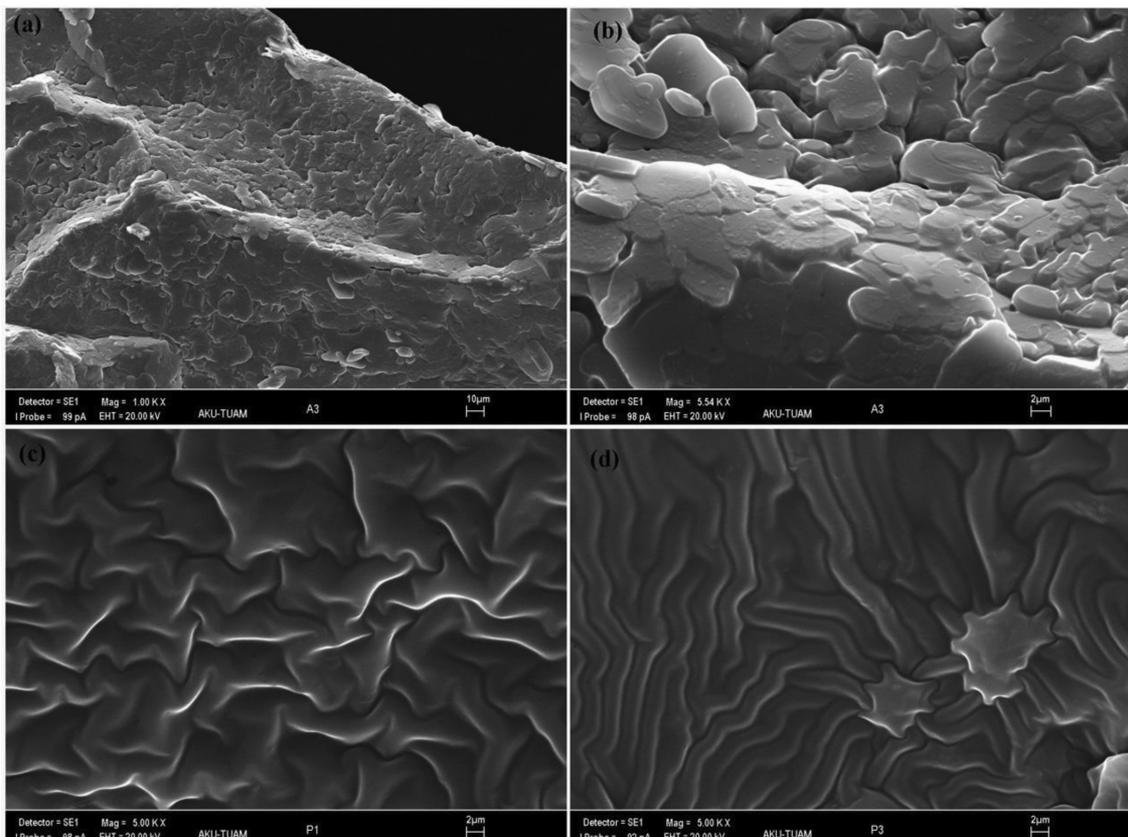
**Figure 2.** SEM images of PEG-DA hydrogels. (a) Surface of 30 % 1000x zoom, (b) Surface of 50 %; 5500x zoom, (c) Section of 30 % 5000x zoom, (d) Section of 50 %; 5000x zoom.
