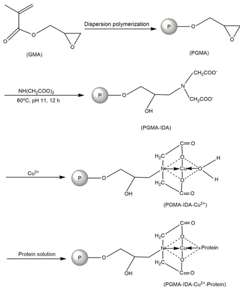
**Figure 1.** Preparation of p(GMA) metal-chelated microspheres.
