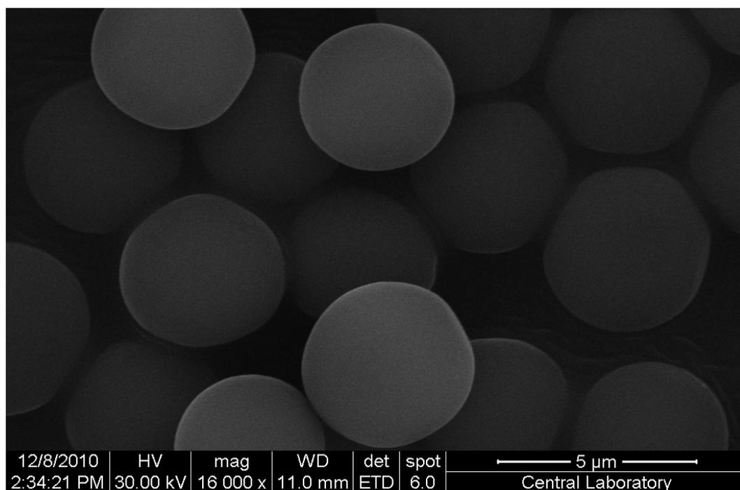
**Figure 2.** SEM image of monosize p(GMA) microspheres.
