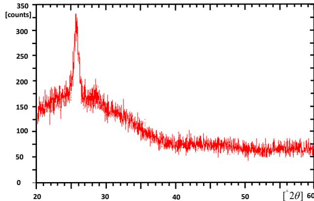
**Figure 1.** XRD spectrum of TiO<sub>2</sub> nanoscale thin films annealed at room temperature.
