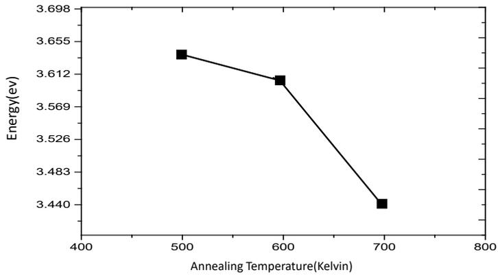
**Figure 6.** The plot of the energy gap in terms of reheating temperature.
