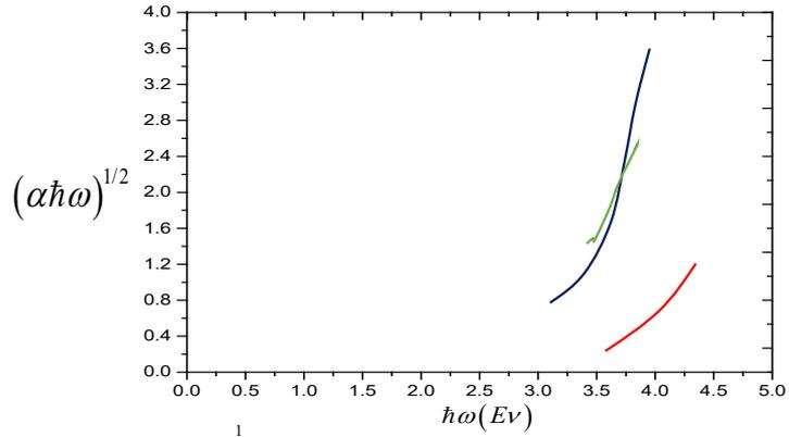
**Figure 5.** Diagram  $\hbar\omega$  based on  $(\alpha\hbar\omega)^{\frac{1}{2}}$ , for sample, prepared by dip - coating after 40 minutes making the solution and at a) 200°C, b) 400°C, C) 600°C are annealed.
