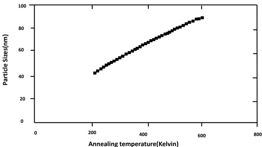
**Figure 4.** Versus of annealing temperature with particles sizes.
