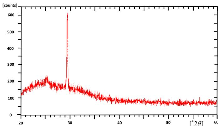
**Figure 3.** XRD spectrum of TiO<sub>2</sub> nanoscale thin films annealed at 400°C.
