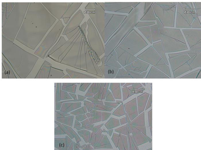
**Figure 8.** The samples prepared by dip-coating method and dried at a) 20°C, b) 100°C and c) 200°C temperature.
