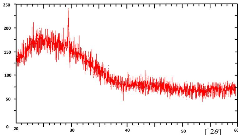
**Figure 2.** XRD spectrum of TiO<sub>2</sub> nanoscale thin films annealed at 200°C.
