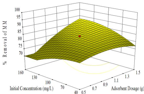
**Figure 7.** 3D response surface plots showing the effect of adsorbent dosage and initial concentration on MB Removal at fixed pH and contact time.
