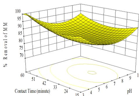
**Figure 4.** 3D response surface plots showing the effect of pH and the contact time on MB removal at fixed adsorbent dosage and initial concentration.
