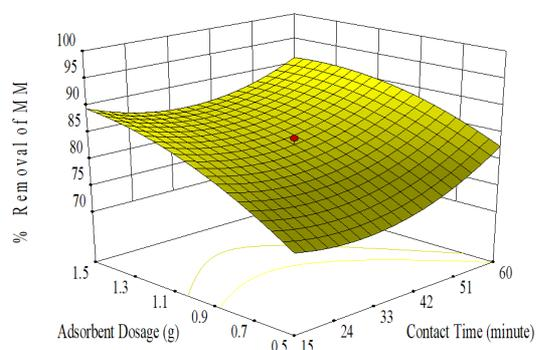
**Figure 6.** 3D response surface plots showing the effect of adsorbent dosage and contact time on MB Removal at fixed pH and initial concentration.
