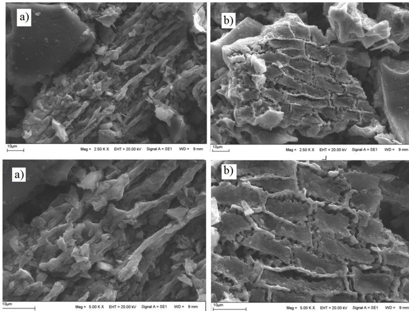
**Figure 3.** SEM image of activated carbon of *Vitis vinifera* seed (a) post-adsorption and (b) pre-adsorption of MB.
