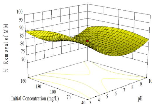
**Figure 5.** 3D response surface plots showing the effect of pH and initial concentration on MB Removal at fixed adsorbent dosage and contact time.
