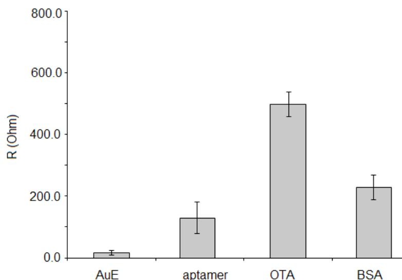
**Figure 4.** Histograms obtained from Rct values in the presence of 5 mM  $[\text{Fe}(\text{CN})_6]^{3-/4-}$  following the experimental procedure detailed in section 2.3 at AuSPCE surfaces under optimum conditions.
