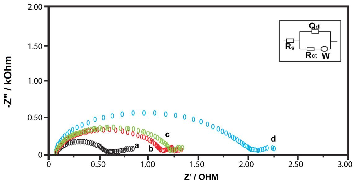
**Figure 2.** Rct values obtained in the presence of 5 mM  $\text{Fe}(\text{CN})_6^{3-/4-}$  at (a) bare, (b) aptamer modified, (c) aptamer-BSA interaction, (d) aptamer-OTA interaction AuSCPE surfaces.
