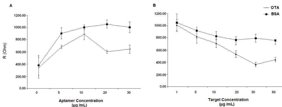
**Figure 3.** Rct values in the presence of 5mM  $[\text{Fe}(\text{CN})_6]^{3-/4-}$  by increasing the concentrations of A) aptamer B) target at aptamer modified surfaces after interaction with OTA target and nonspecific BSA molecules.
