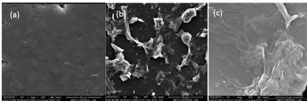
**Figure 2.** SEM images of bare GCE (a) and GCE/ERGO/P(PDCA) (b,c)
