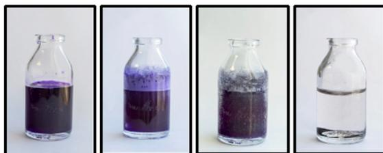
**Figure 3.** Progressive decolorization of CV solution in 20 min with the  $\text{MnO}_2/\text{H}_2\text{O}_2$  catalyst.
