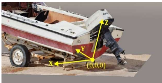
Fig. 13. Coordinate center of the 3D model
