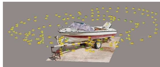
Fig. 3. Camera stations configuration of the boat
