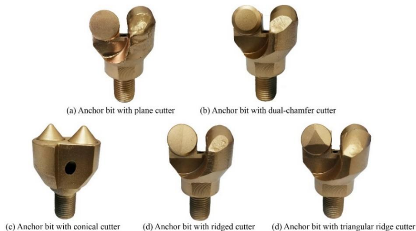
Figure 14. Anchor bits with special-shaped PDC cutters
