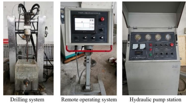
Figure 13. Main components of micro-drilling test device
