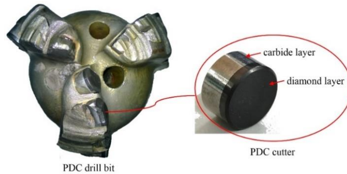
Figure 1. PDC drill bit wear photo
