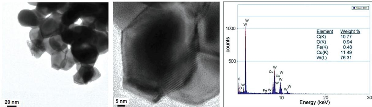
Figure 8. TEM images of  $W_2B$  nanocrystals after leaching
