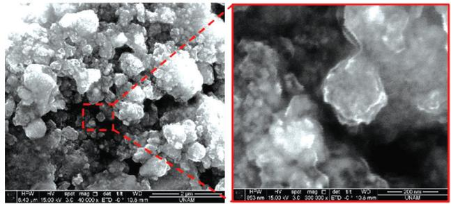
Figure 7. SEM images of  $\text{W}_2\text{B}$  nanocrystals after leaching
