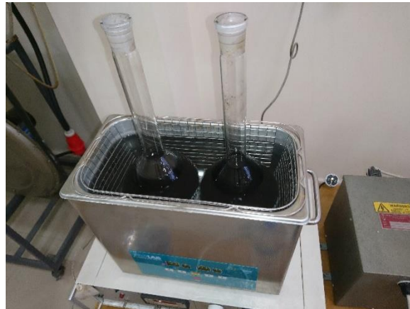
Figure 1. Hybrid nanofluid held in an ultrasonic bath
