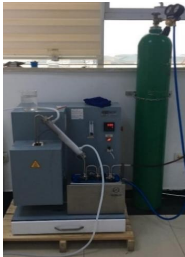
Figure 2. Fixed bed carbonization reactor and its schematic view.
