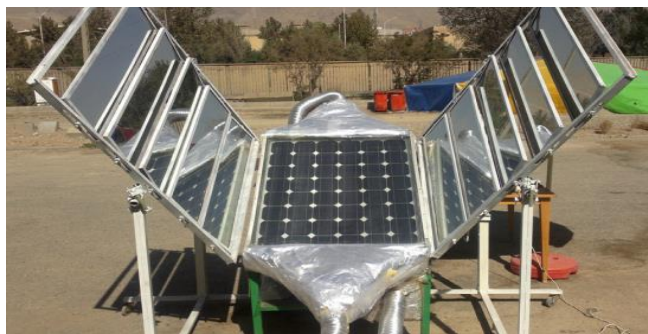
Figure 17. The PV/T collector and Fresnel reflector [56].
