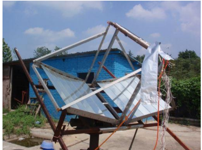
Figure 3. Experimental set-up of water-cooled CPV module [23].
