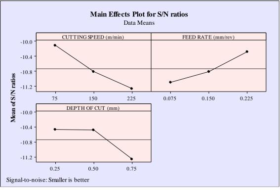
Figure.4. Optimum cutting parameters for minimum energy consumption
