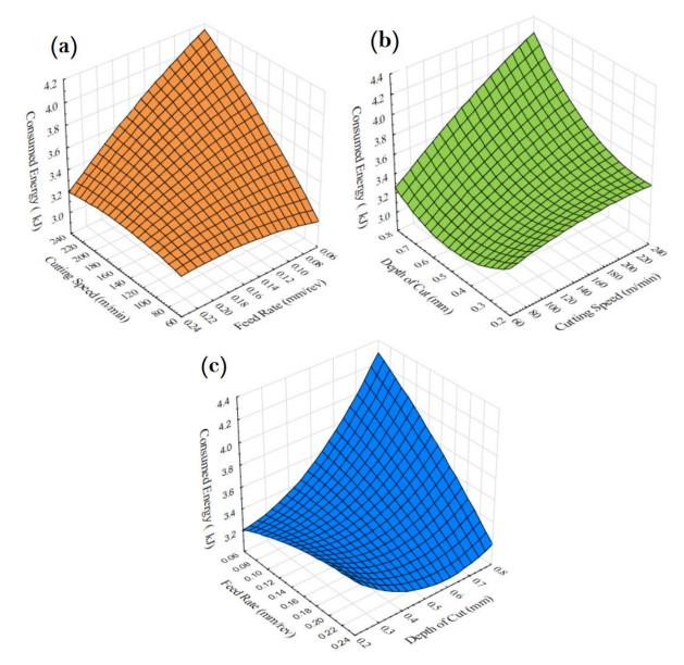
Figure.3. 3D plots for the combined effect of cutting parameters on energy consumption
