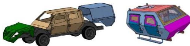
**Fig.2.** Concept Design: The main part separation and personnel cabin details
