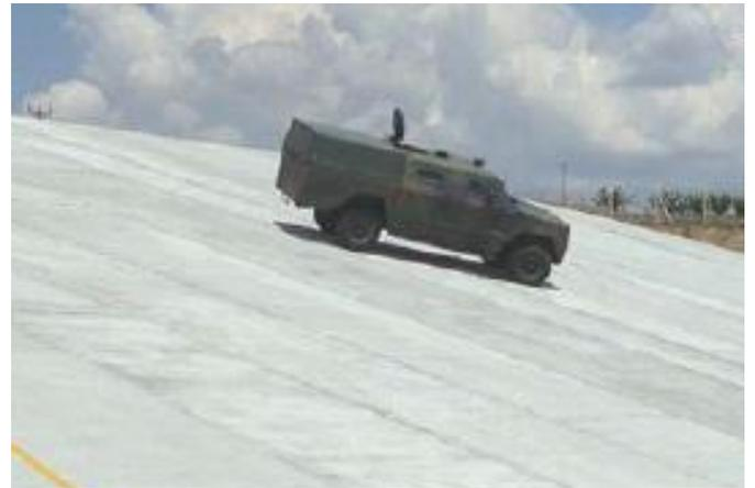
Fig. 9. Side slope performance test of GEKKO.
