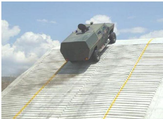
Fig. 8. Climbing performance test of GEKKO.
