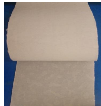
Figure 8. Image of the enzyme treated double-layered coated UV-cured fabric sample after peel test.
