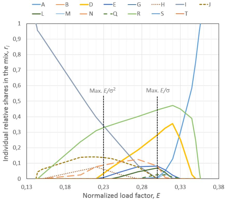
Figure 8. Solutions of the optimization problem for 15 Croatian wind plant sites, using the 15-minute readings during the entire 2018. Source: authors' calculation.
