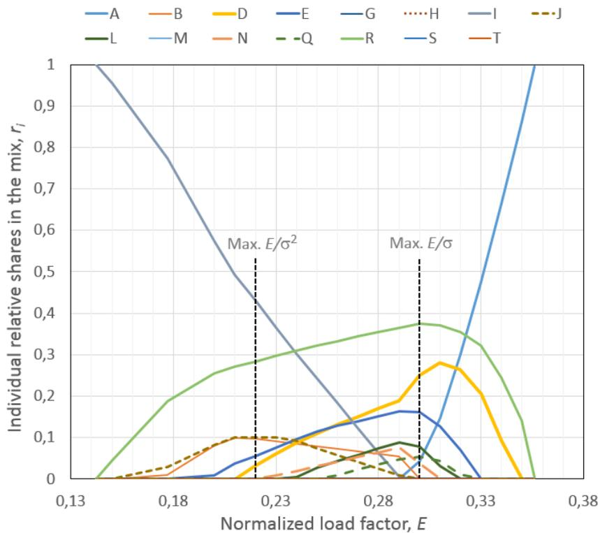
Figure 9. Solutions of the optimization problem for 15 Croatian wind plant sites, using the 15-minute readings during the entire 2017. Source: authors' calculation.
