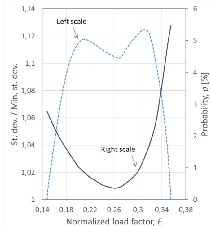
Figure 13. The probability that the hourly change in production will exceed 20% of total capacity and the ratio between the actual and minimum possible standard deviation. Source: Authors.
