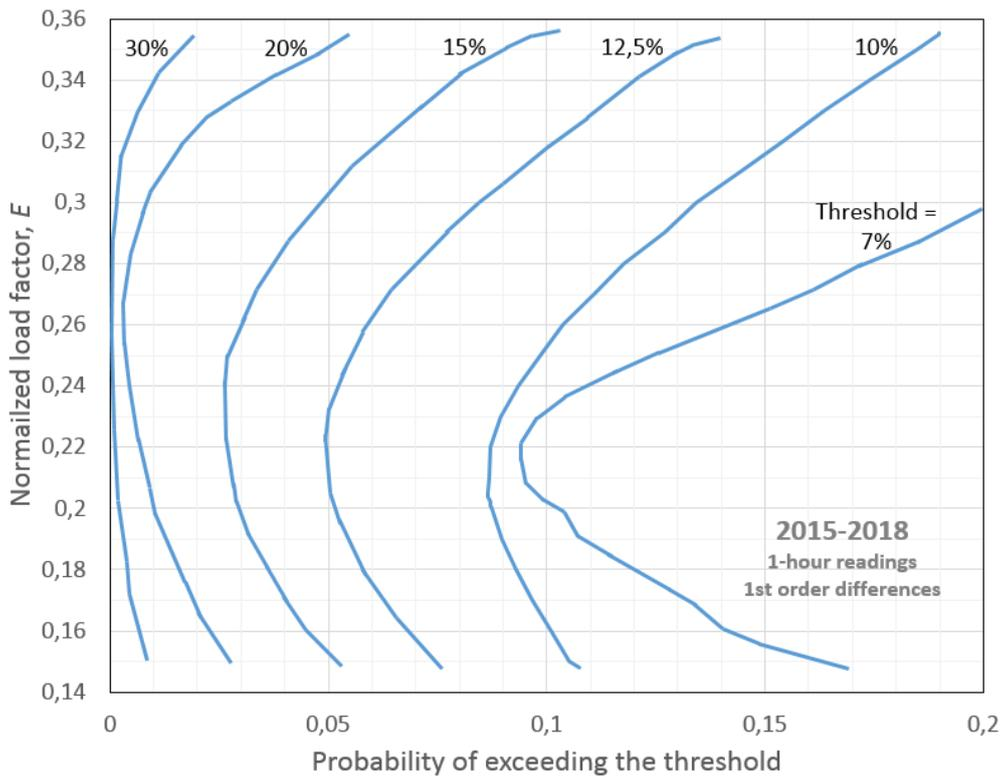
Figure 11. Efficient frontiers where the probability of a one-hour change (1<sup>st</sup> order difference) in total normalized production exceeding the Threshold is minimized for any given  $E$ . Derived from the 4-year time series of 1-hour readings, 2015-2018. Source: authors' calculation.
