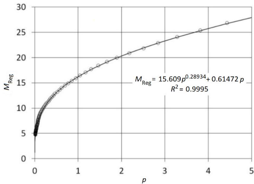
Figure 10. Experimentally obtained demand for fast regulation and the best-fit function (2). Source: [16].
