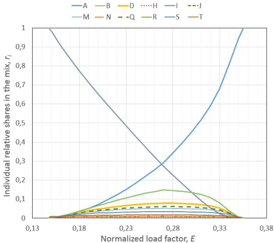
Figure 12. Solutions of the optimization problem along the curve for the Threshold = 20% from Fig. 11. Source: authors' calculation.
