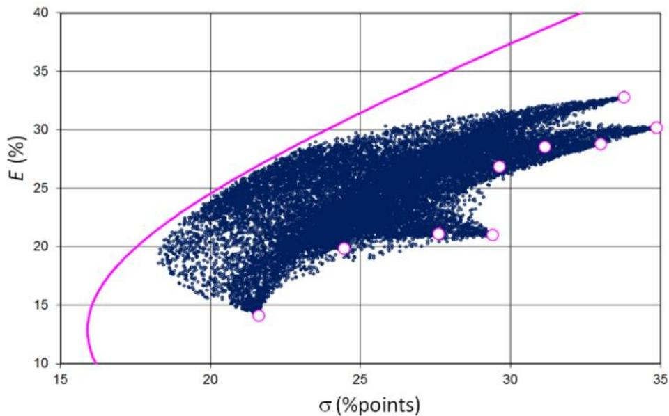
Figure 4. Small dots: 20 thousand random portfolios made with nine then active wind plants, based on 2014 15-minute data. Source: [1].
