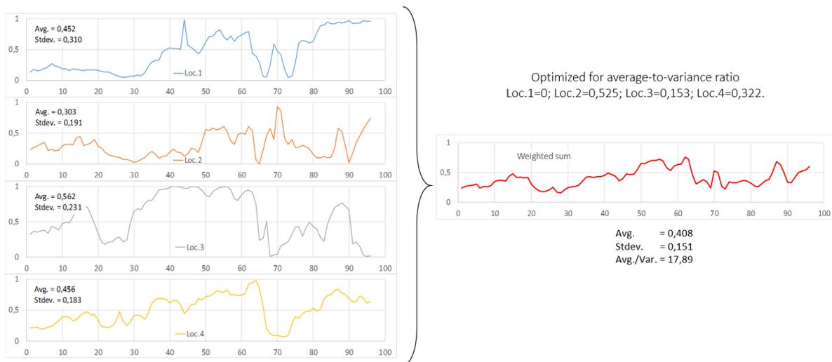
Figure 1. The measured normalized wind generation time series at four locations in 24 hours combined for maximized Average-to-Variance ratio. Source: Authors
