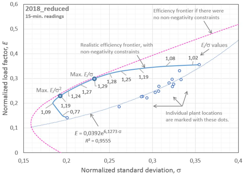
Figure 6. Efficient frontiers derived from the data for 15 Croatian wind plant sites, using the 15-minute readings from the entire 2018. Source: authors' calculation.
