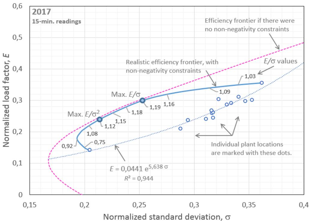
Figure 7. Efficient frontiers derived from the data for 15 Croatian wind plant sites, using the 15-minute readings from the entire 2017. Source: authors' calculation.
