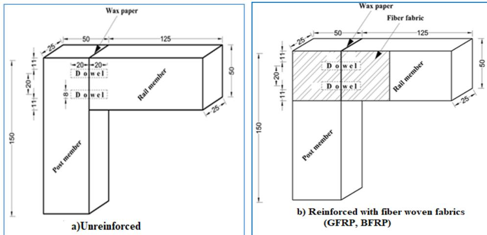
Figure 2: General configuration of L-shaped joint specimens (dimensions in mm)
