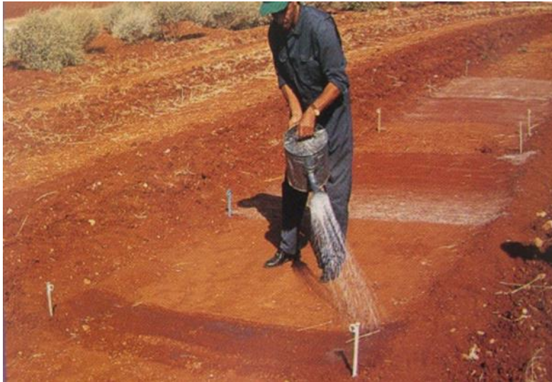
Figure 8. Paraffin Application Providing Impermeability on the Soil Surface
