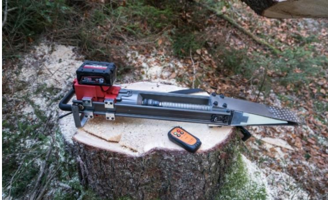
Figure 2. Remote controlled felling wedge Forstreich TR300
