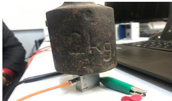
Figure 2. Test of the load cell
