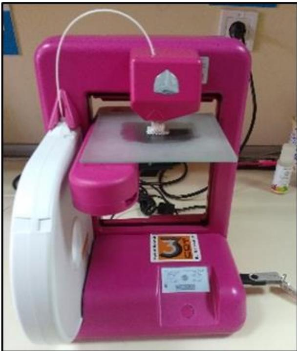
**Figure 1.** Picture of the 3D Systems Cube 2<sup>nd</sup> generation 3d printer
