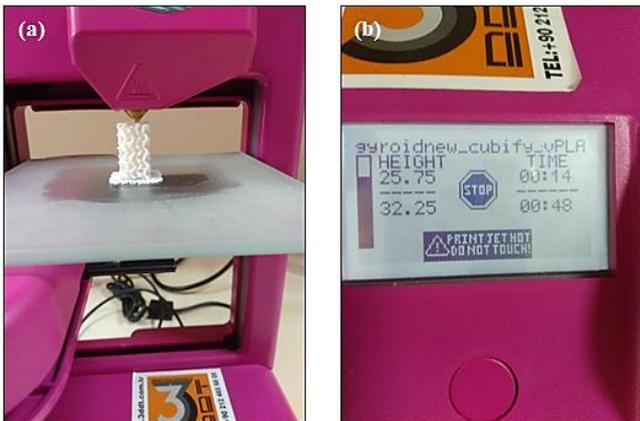
**Figure 4.** Pictures of (a) the 3d printing process of the PLA scaffold and (b) the screen view of the 3d printer during the printing procedure
