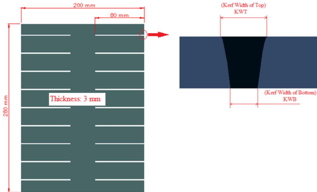
**Figure 1.** Workpiece dimensions, kerf width of top and kerf width of bottom
