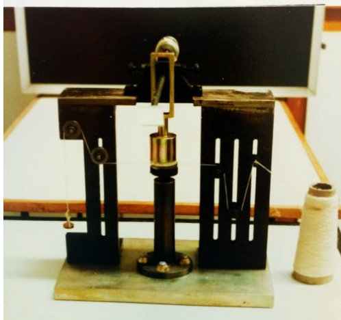
Figure 17. Yarn compression Measuring apparatus: Side view [17]
