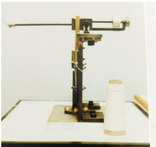
Figure 16. Yarn compression Measuring apparatus: Top view [17]
