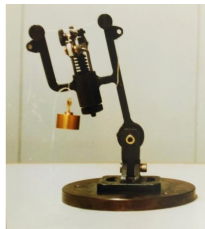
Figure 24. Yarn compression measuring apparatus in weaving conditions [17]
