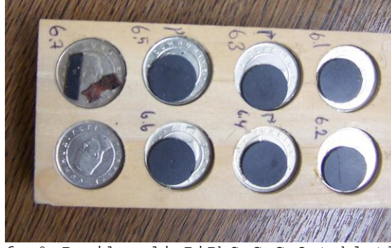
Şekil 6. % Zn ilaveli BiPbSrCaCuO tabletler[20] (Figure 6. Pellets of added Zn% in to BiPbSrCaCuO)
