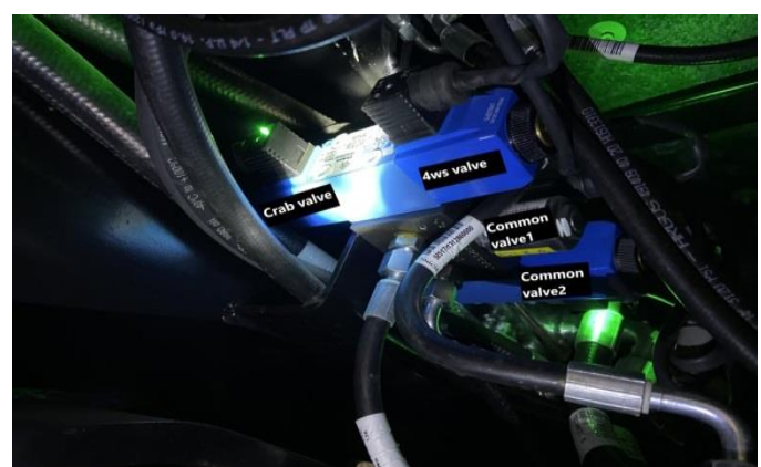
Fig.12. Condition of valves in crab rotation mode
