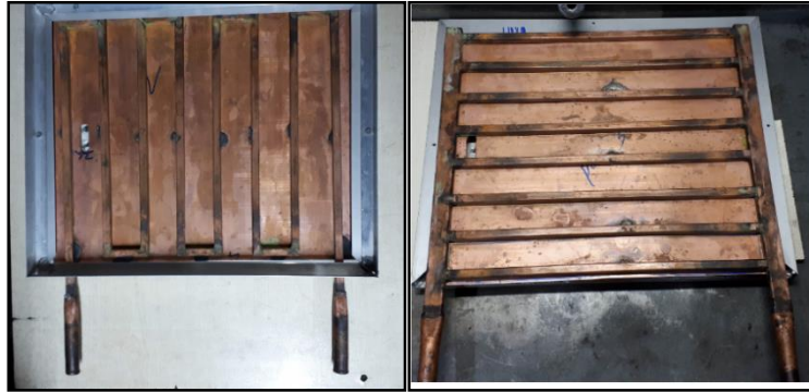
Figure 2. Serpentine, head and riser heat exchanger designs
