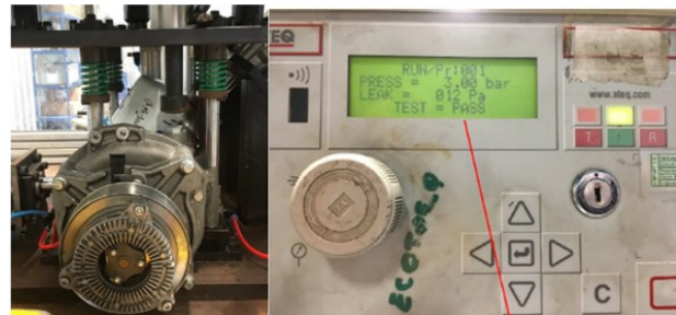
Figure 4. Leakage Test and Results
